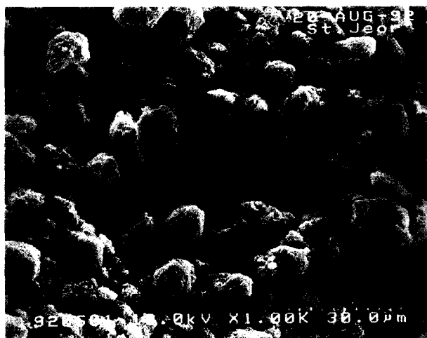
Figure 7 FESEM micrograph of urea-terminated poly(1,6-hexamethyleneurea) synthesized at 185°C
